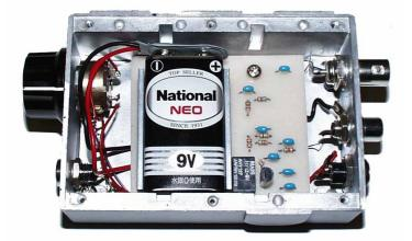
If using an external power supply, keep the power supply as far away from the WL500 and receiver as practical to reduce noise. If using the optional 500LM element, you may wish to consider use of a low noise regulated
