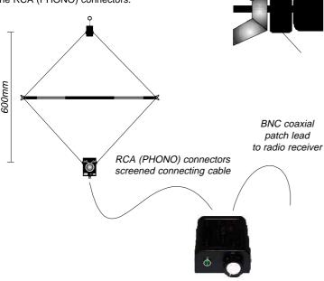
**3.** Connect the BNC-BNC coaxial patch lead between the 'RX' socket of the control box and short wave radio receiver (if your radio cannot accommodate a BNC plug, use an inter-series adapter).
